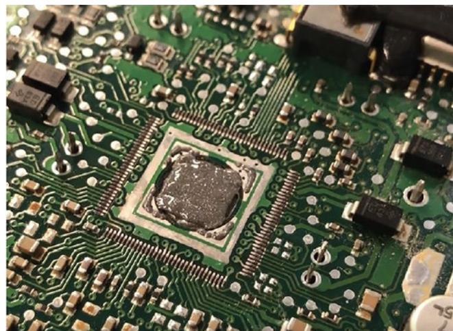
Figure 10: Complete TQFP after jetting.
