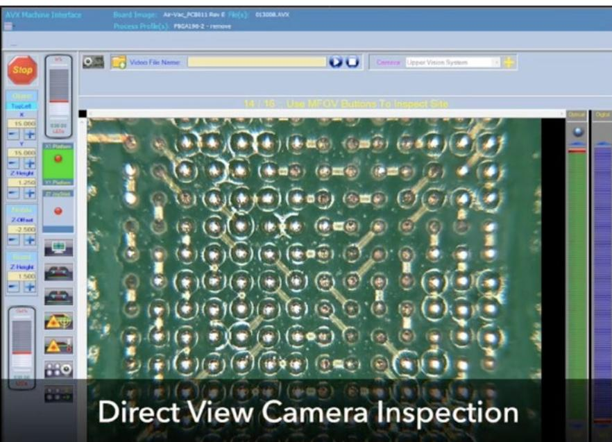
coplanarity and depth while gradually approaching an appropriate depth above the pads. The remnant solder becomes the pre-tinned pad for the replacement component.
