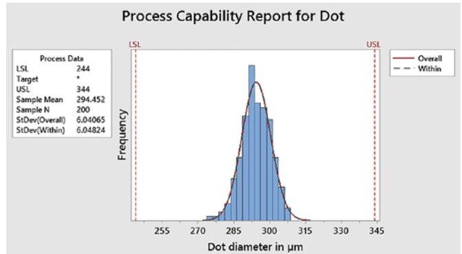
Figure 13: Dot diameter distribution of the BGA component.
