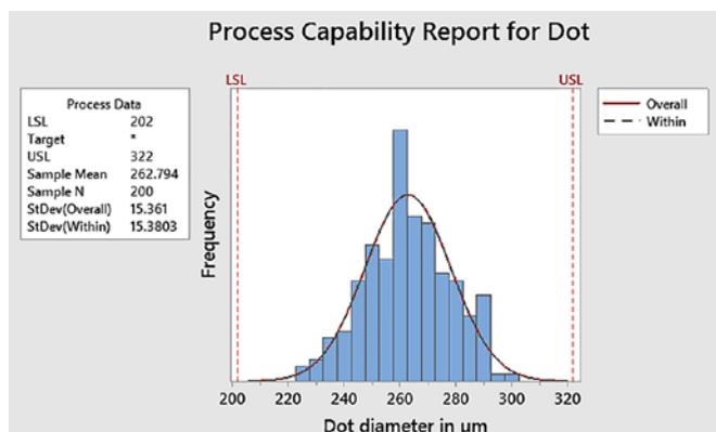
Figure 5: Dot diameter distribution in Zone A.
