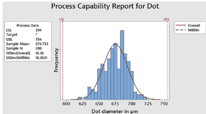
Figure 9: Dot diameter distribution in zones B and C.
