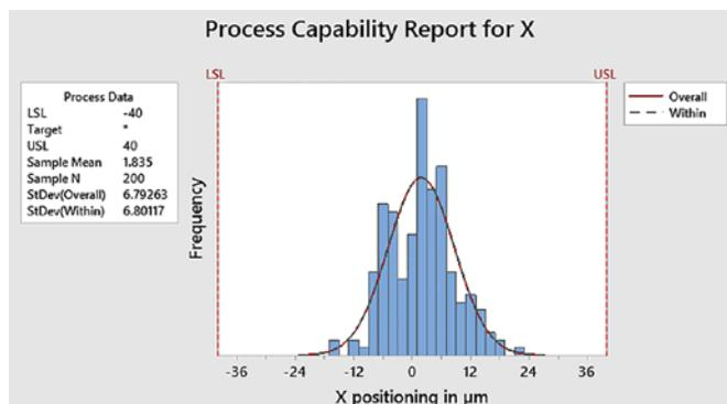
Figure 3: Distribution of the X positioning in Zone A.
