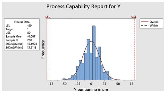
Figure 8: Distribution of the Y positioning in zones B and C.
