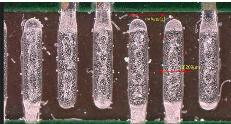
Figure 6: 400 µm pitch after jetting.
