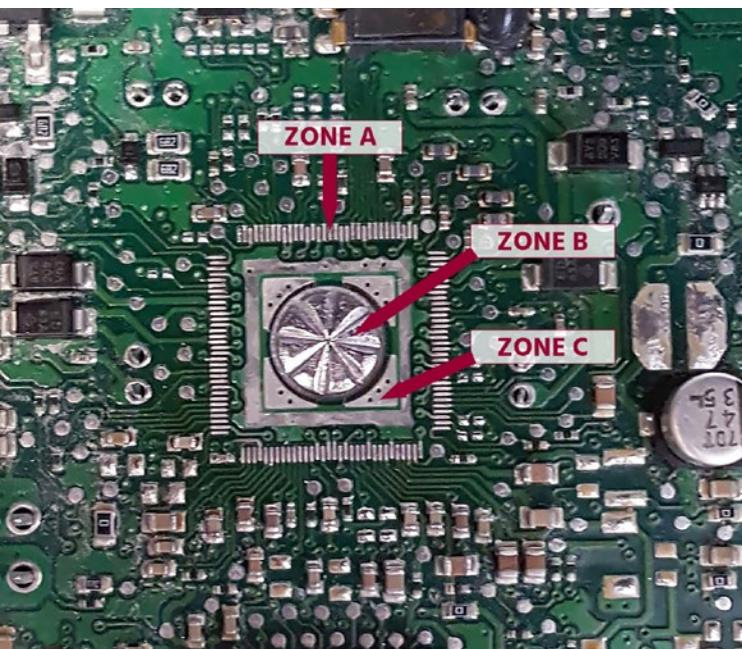
Figure 1: Component to be repaired, TQFP (thin quad flat package).
