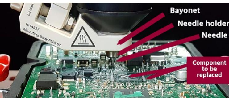
Figure 2: Needle, needle holder, and bayonet.
