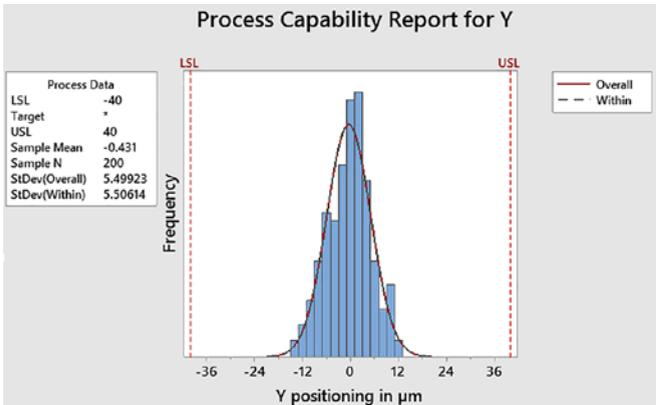
Figure 12: Distribution of the Y positioning of the BGA component.
