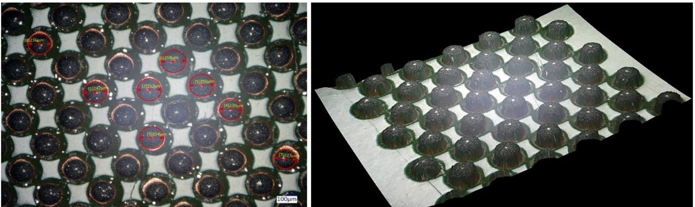
Figure 14: BGA component after jetting.
