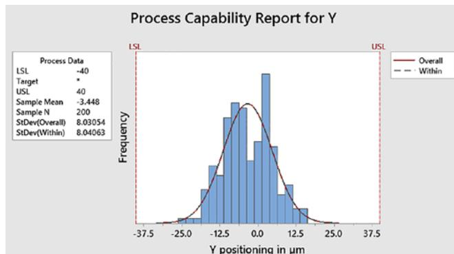
Figure 4: Distribution of the Y positioning in Zone A.
