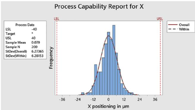
Figure 11: Distribution of the X positioning of the BGA component.
