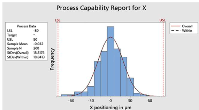
Figure 7: Distribution of the X positioning in zones B and C.
