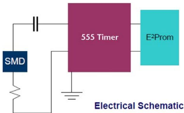
Figure 9: Electrical schematic of circuit to detect capacitor change (capacitor is strain monitoring device, or SMD).
