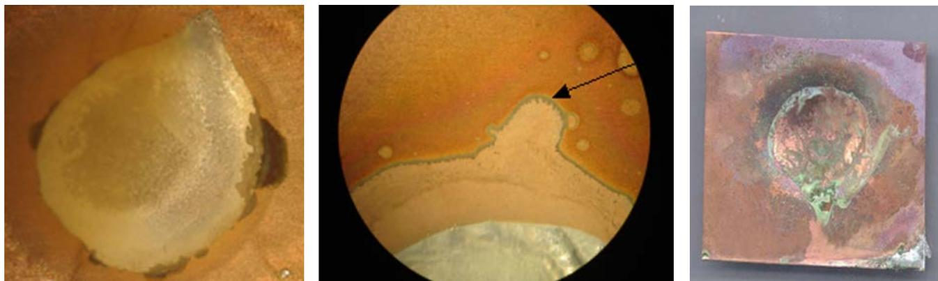
Figure 2: Corrosion test showing (l-r) no corrosion, minor corrosion and major corrosion.
