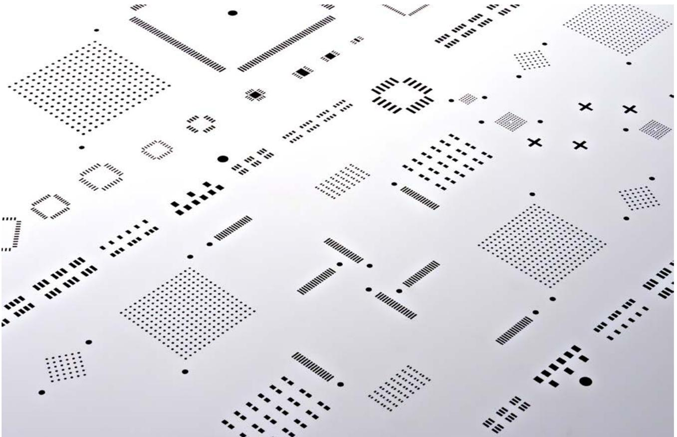
Figure 1: Standard electroformed stencil image.
