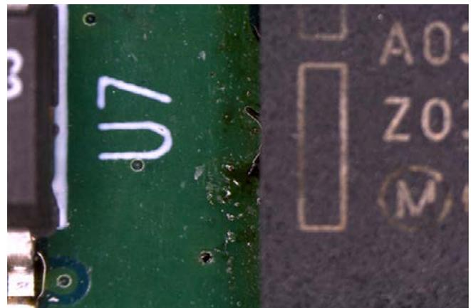
Figure 8: Excessive flux residue observed surrounding BGA.
