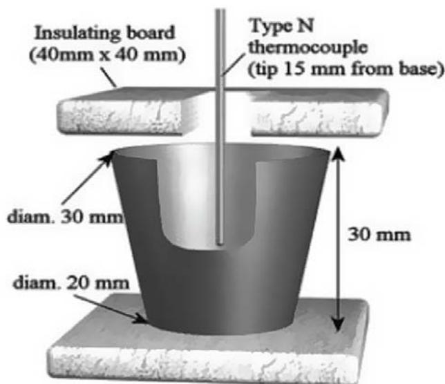
Figure 3. Thermal analysis set-up.
