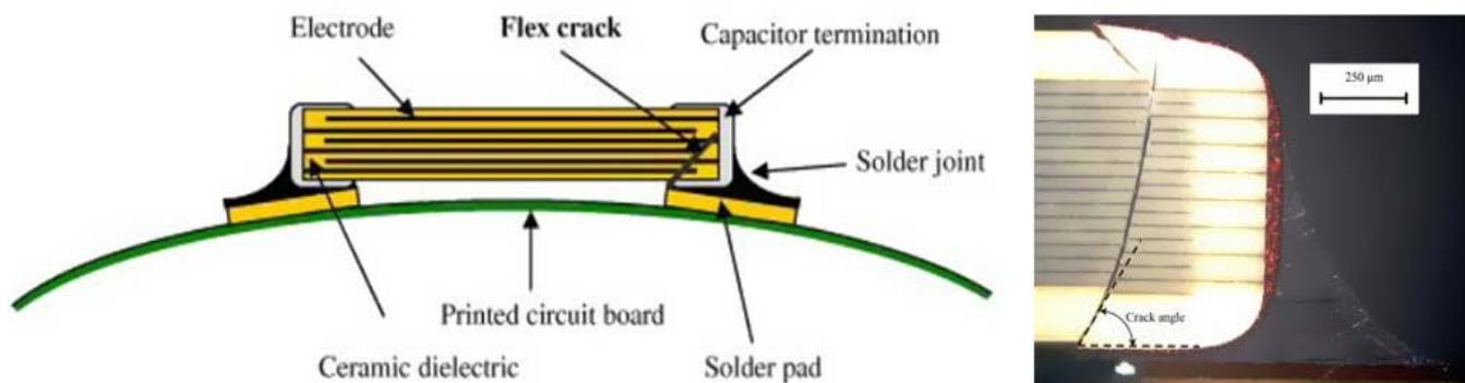
Figure 10: Typical crack signature of chip capacitor under flexural loading<sup>[8]</sup>.
