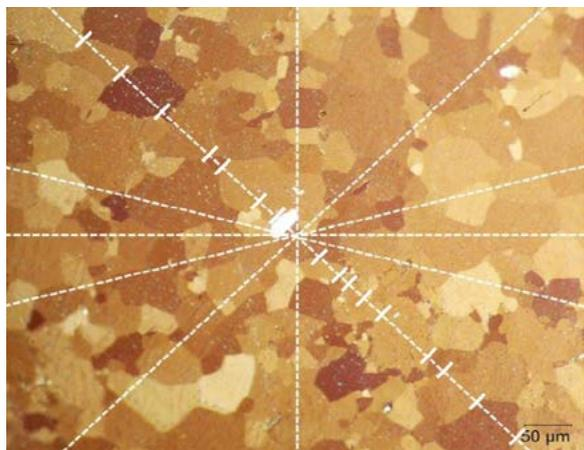
Figure 6: Intercepts along which the recrystallized tin grain were counted in cross sections.
