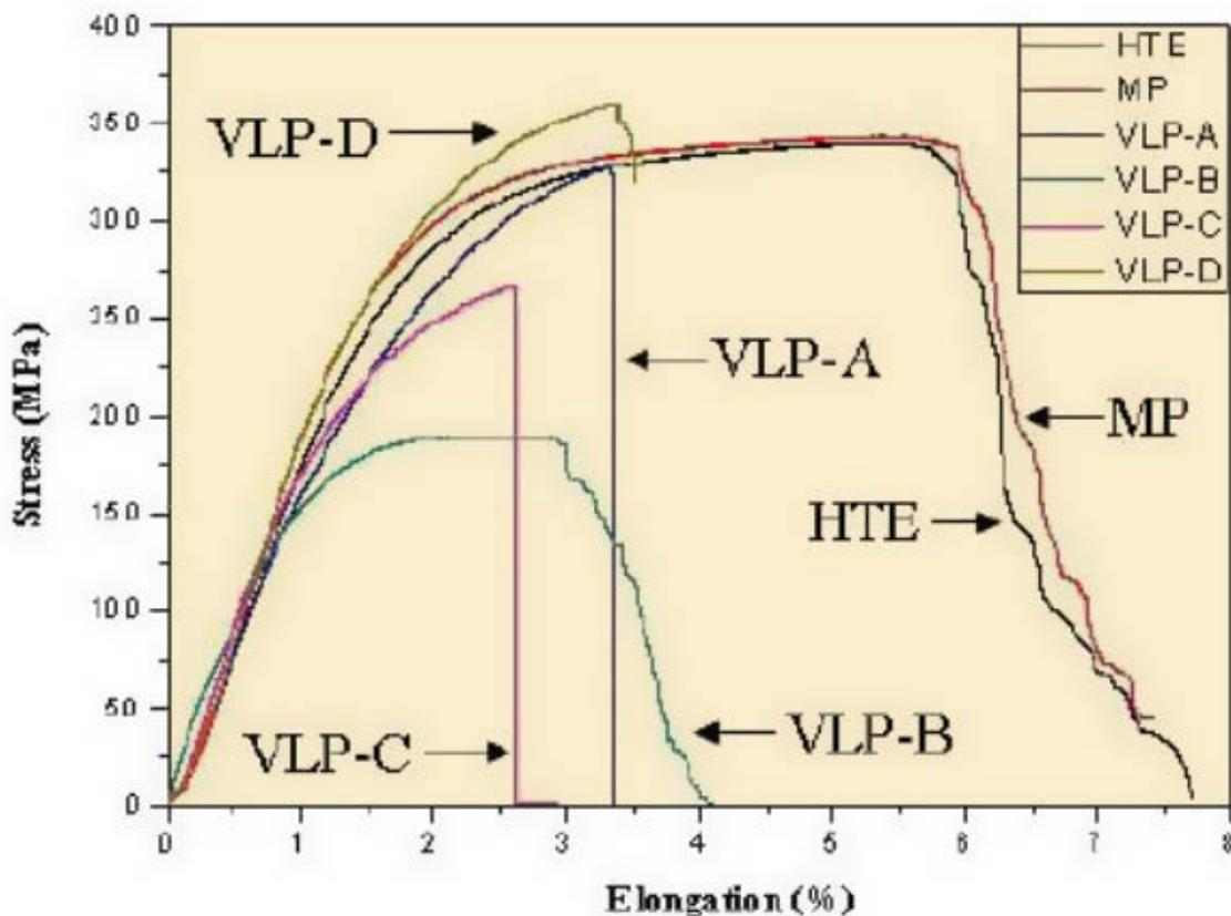
Figure 7: Stress/strain curve of different PCB copper trace materials. The most commonly used is high-temperature electrolytic (HTE)<sup>[5]</sup>.
