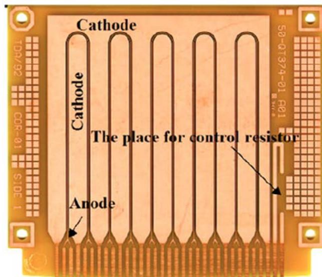
Figure 5: Modified Bono test pattern.
