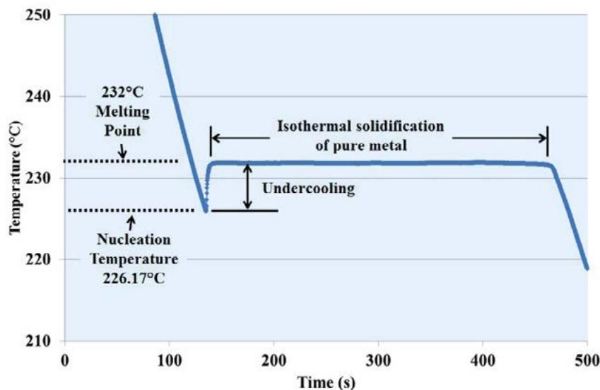
Figure 1: Cooling curve for pure tin showing the undercooling required to trigger nucleation of solid.
