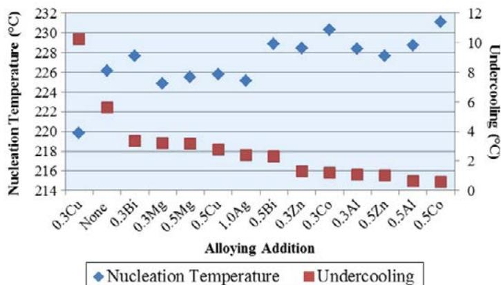
Figure 7: The effect of composition on nucleation temperature and undercooling with the results presented in order of decreasing undercooling.
