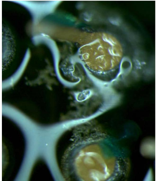
Figure 10: Excessive flux residue and dendritic growth visible once BGA component was removed.
