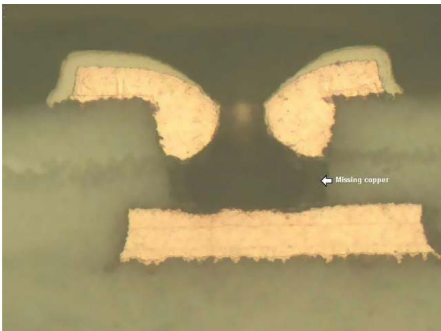
Photo 12: Blind via with missing copper plating.
