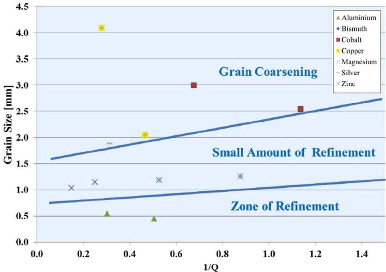
Figure 10: Relationship between the grain and the reciprocal of diffusion rate of solute atoms in the liquid at the solid liquid interface (the growth restriction factor).
