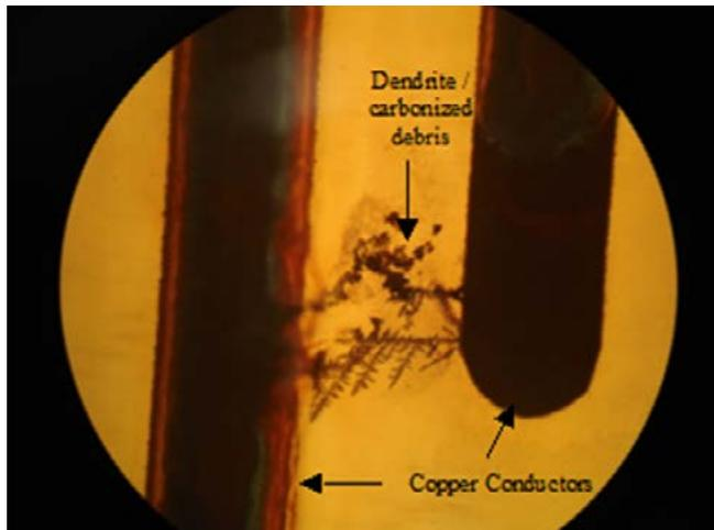
Figure 7: Carbonized debris.
