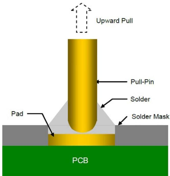
Figure 2: Test setup schematic<sup>[4]</sup>.
