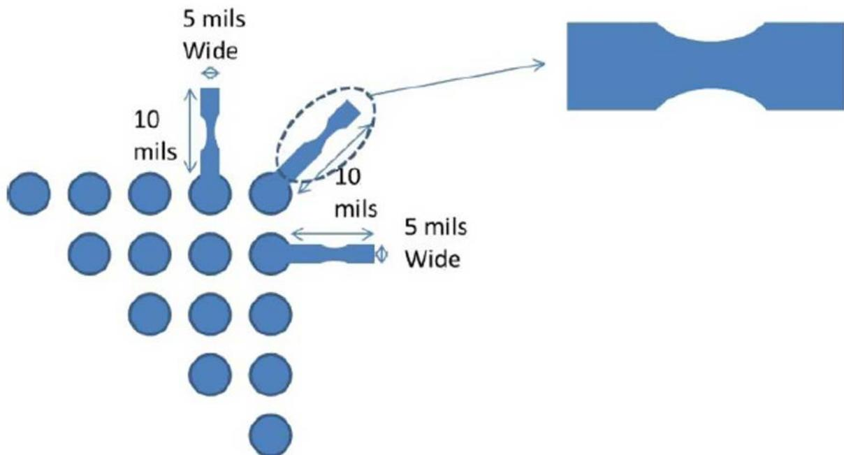
Figure 6: “Mousebite” trace design to fail at preset strain threshold.
