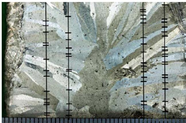
Figure 5: Intercept counting method used to characterize the size of as-cast grains.
