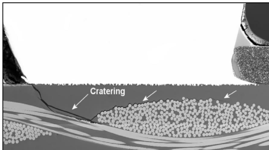
Figure 1: Example of a pad cratering failure<sup>[4]</sup>.
