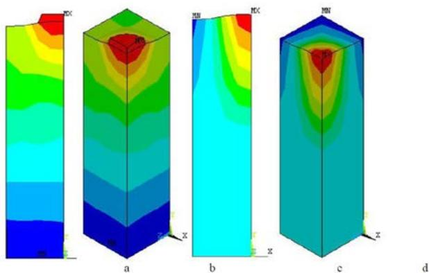
Figure 4: Numerical analysis results: (a) vertical deformation, front view; (b) vertical deformation, isometric view; (c) vertical tensile ( $s_y$ ) stress, front view; (d) vertical tensile ( $s_y$ ) stress, isometric view.
