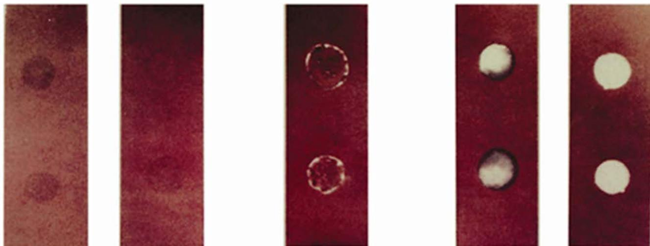
Figure 1: Copper mirror test. L = no breakthrough, M = less than 50% breakthrough, H = greater than 50% breakthrough.
