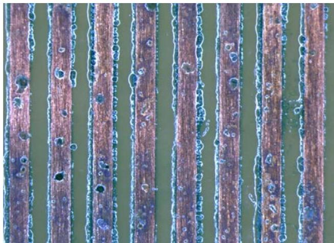
Figure 3: Flux corrosion of copper conductors.
