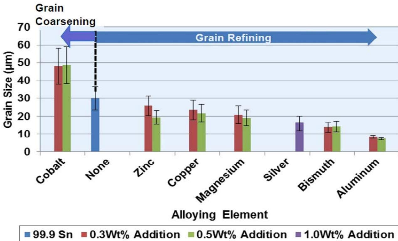
Figure 9: Effect of alloying addition on the recrystallized tin grain size. Results ranked by grain size with 0.3 Wt% addition with results for pure tin and silver interpolated.
