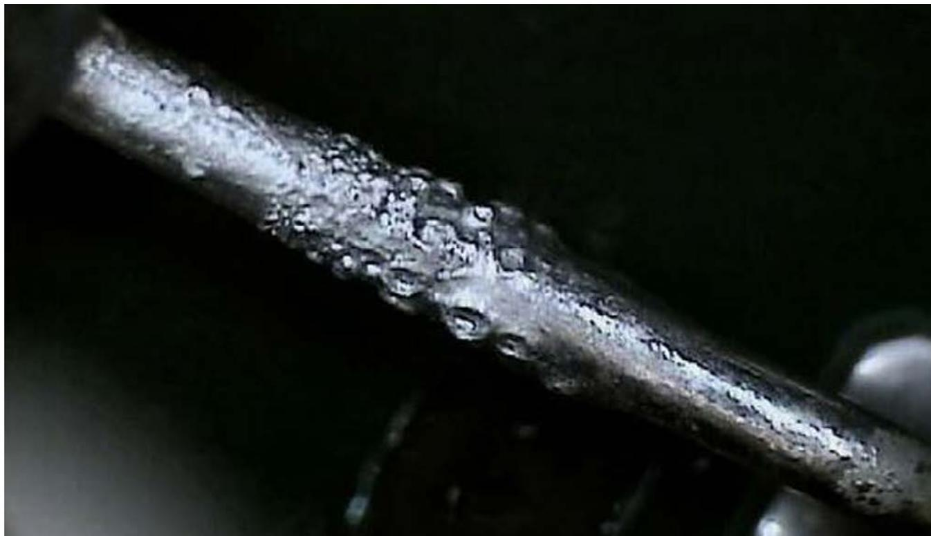
Figure 1: An acid bright dip can lead to blistering after heat exposure. (Photo courtesy of David Hillman, Rockwell Collins)
