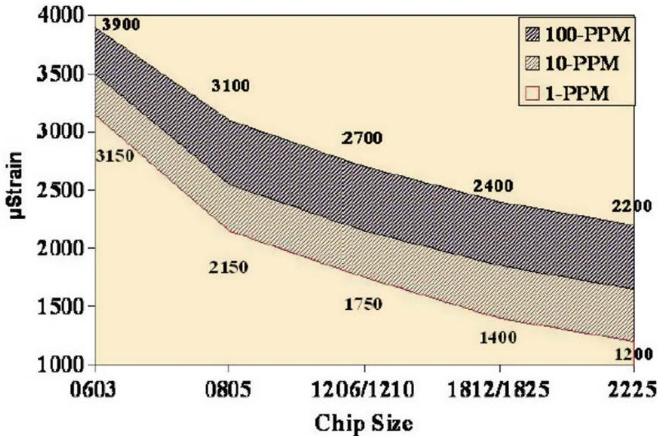
Figure 8: Chip size versus strain required to achieve 100, 10, and 1 ppm failure rates (typical)<sup>[7]</sup>.
