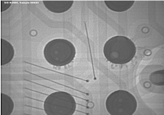
Figure 9: X-ray image showing dendritic growth beneath BGA.
