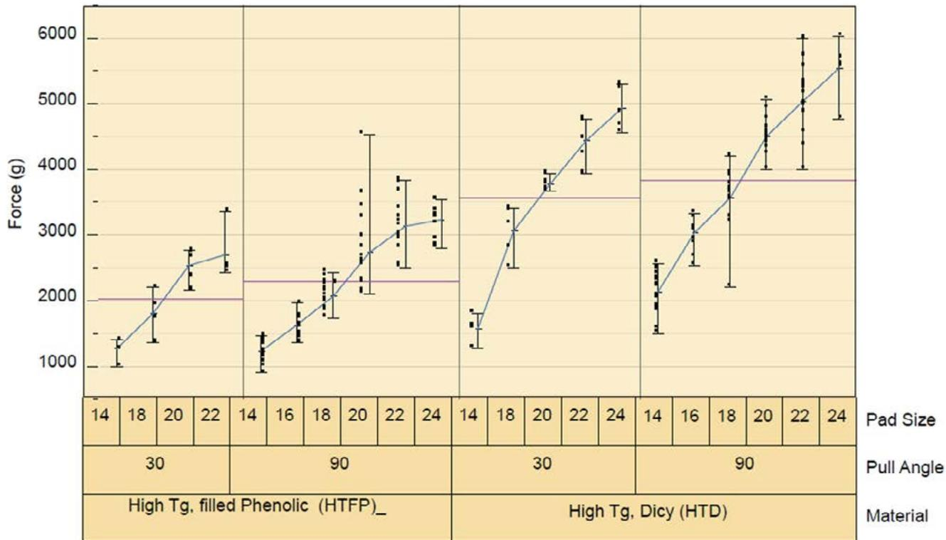
Figure 3: Effect of pull angle (5 mil stencil, 5 mm/sec pull speed, 500 μm pin size)<sup>[4]</sup>.
