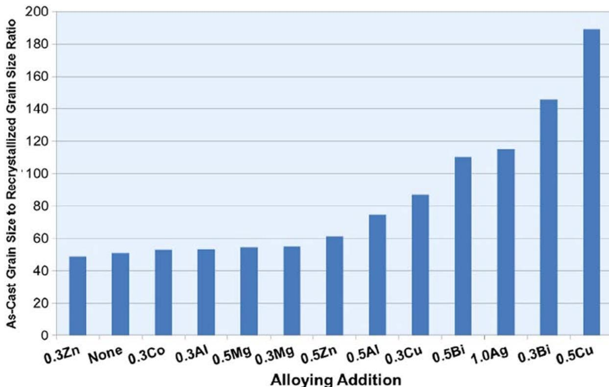
Figure 11: Ratio of as-cast to recrystallized grain size as a function of alloy.
