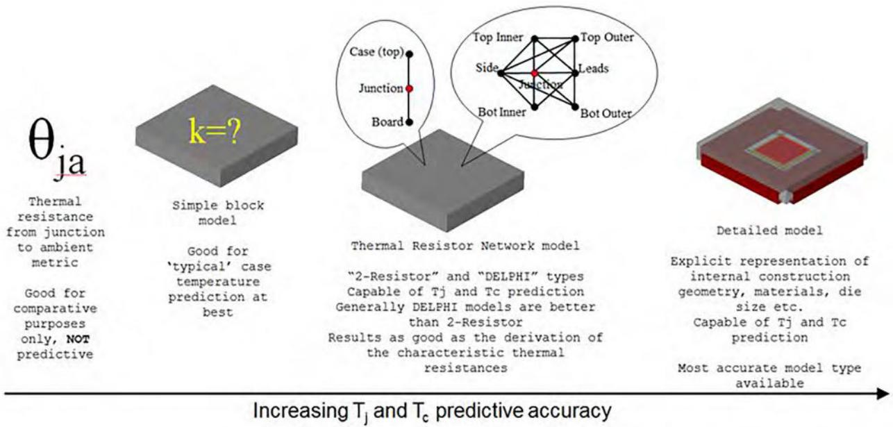
Figure 2: Hierarchy of package thermal information for design.
