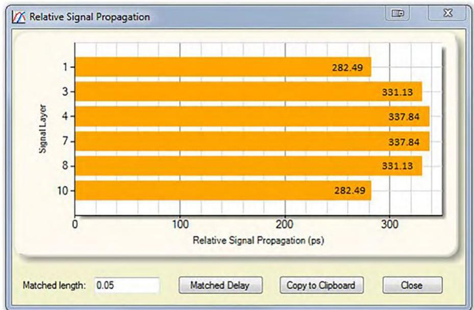
Figure 3: Relative signal propagation of microstrip and stripline, simulated in iCD Design Integrity.
