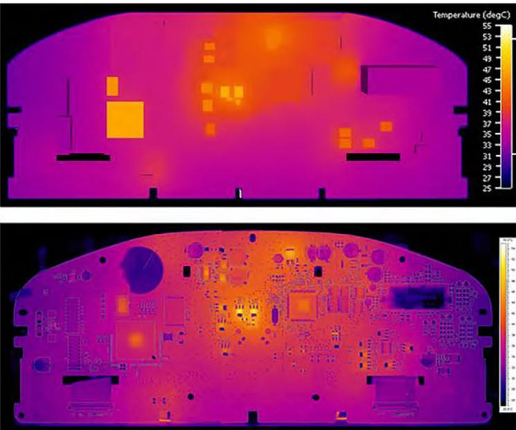
Figure 3: Thermal simulation modeling result (top), compared with a PCB measured using an IR camera (bottom).
