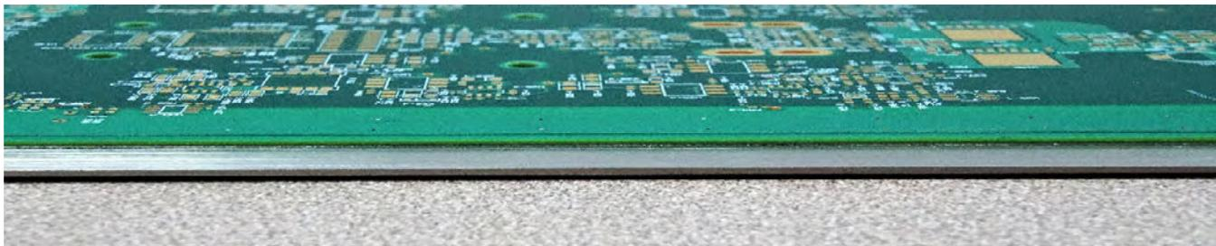
Figure 7: Milling on a metal core PCB.
