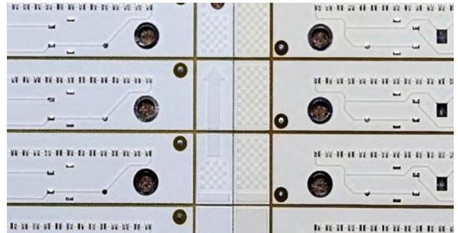
Figure 3: Solder mask "browning" with multiple reflow cycles.
