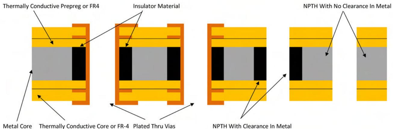
Figure 6: Schematic of a multilayer metal core board.
