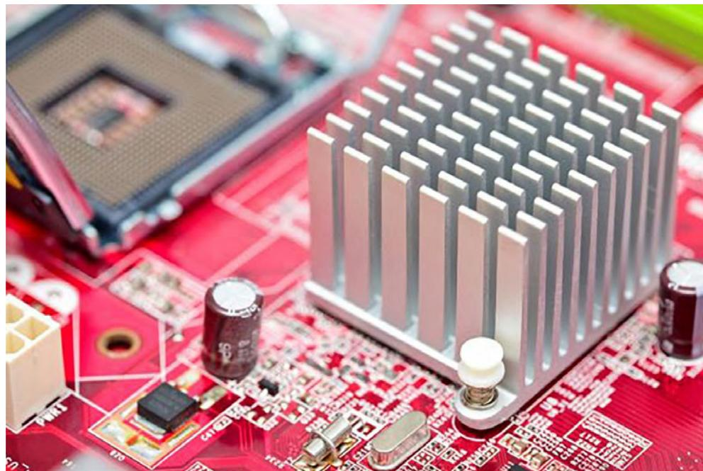
Figure 1: Heatsink with retaining pins that extends beyond the package body.
