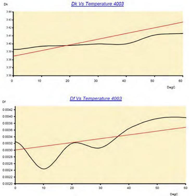
Figure 4: Dielectric constant vs. temperature (top), and dielectric loss vs. temperature (bottom). Source: Rogers Corporation
