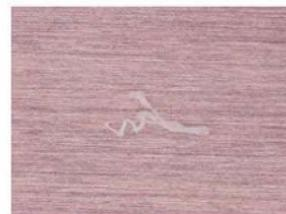
Figure 17: Microscopy image of de-wetting at the SOT solder joint and visual image of foreign object debris.
