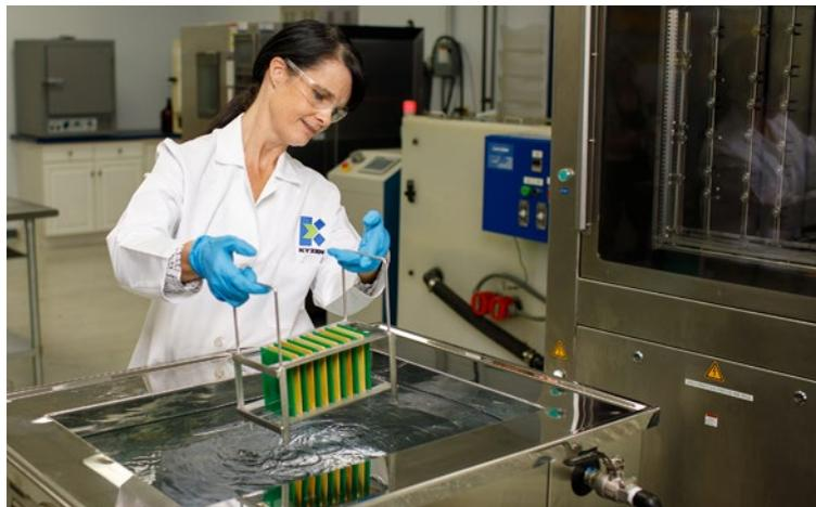
Ultrasonic cleaning ensures the cleaning agent reaches every surface of the circuit boards.
